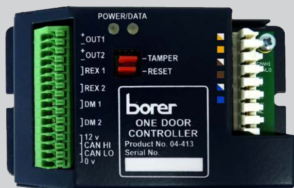
One/Two Door Lock Manager Size: 82 x 45 x 19 mm
